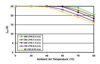
Figure 7: Maximum output power derating curves vs. ambient air temperature for airflow rates of 50 LFM through 400 LFM with air flowing from pin 3 to pin 1 (48V input).
