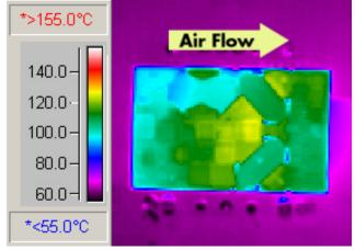
Figure 12: Therrmal plot of converter at 24 amp load current with 55°C air flowing at the rate of 200 LFM. Air is flowing across the converter from input to output (48V input).
