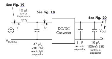
Figure 17: Test set-up diagram showing measurement points for Input Terminal Ripple Current (Figure 18), Input Reflected Ripple Current (Figure 19) and Output Voltage Ripple (Figure 20).
