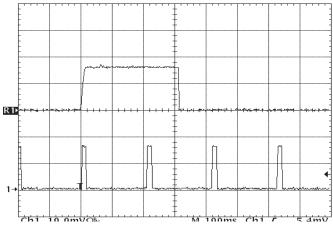
Figure 22: Load Current (20A/div) as a funtion of time when the converter attempts to turn on into a 10 m $\Omega$  short circuit. Top trace (5ms/div) is an expansion of the on-time portion of the bottom trace.
