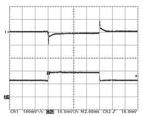
Figure 15: Output voltage response to step-change in load curent (50%-75%-50% of Iout(max);  $dI/dt = 0.1A/\mu s$ ). Load cap:  $10\mu F$ ,  $100 \text{ m}\Omega$  ESR tantalum cap and 1µF ceramic cap. Ch 1: Vout (100mV/div), Ch 2: Iout (10A/div).
