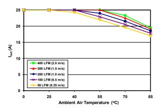
Figure 11: Maximum output power-derating curves vs. ambient air temperature for airflow rates of 50 LFM through 400 LFM with air flowing from input to output (48V input).
