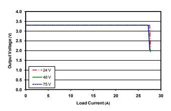
Figure 21: Output voltage vs. load current showing typical current lmit curves and converter shutdown points.
