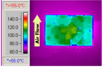
Figure 6: Thermal plot of converter at 25 amp load current with 55°C air flowing at the rate of 200 LFM. Air is flowing across the converter from pin 3 to pin 1 (24V input).
