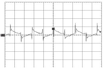
Figure 20: Output voltage ripple at nominal input voltage and rated load current (20 mV/div). Load capacitance: 1µF ceramic capacitor and 10µF tantalum capacitor. Bandwidth: 20 MHz. See Figure 17.
