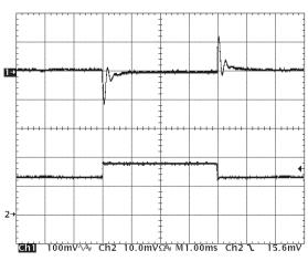
Figure 16: Output voltage response to step-change in load current (50%-75%-50% of Iout(max):  $dI/dt = 5A/\mu s$ ). Load cap 470 $\mu F$ , 30 m $\Omega$  ESR tantalum cap and 1µF ceramic cap. Ch 1: Vout (100mV/div), Ch 2: Iout (10A/div).
