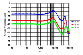
Figure 25: Magnitude of invremental reverse transmission (RT = Iin/Iout) for minimum, nominal, and maximum input voltage at full rated power.
