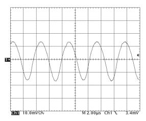
Figure 18: Input Terminal Ripple Current, ic, at full rated output current and nominal in put voltage with 10µH source impedance and 47µF electrolytic capacitor (200 mA/div). See Figure 17.
