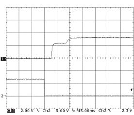
Figure 14: Turn-on transient at zero load (5 ms/div). Ch 1: Vout (2V/div). Ch 2: ON/OFF input (5V/div).
