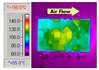
Figure 10: Thermal plot of converter at 24 amp load current with 55°C air flowing at the rate of 200 LFM. Air is flowing across the converter from input to output (24V input).
