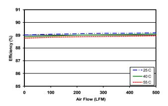
Figure 2: Efficiency at nominal output voltage and 60% rated power vs. airflow rate for ambient air temperatures of 25°C, 40°C and 55°C (48V input).
