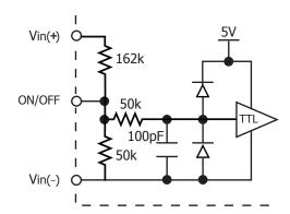
Figure B: Internal ON/OFF pin circuitry
