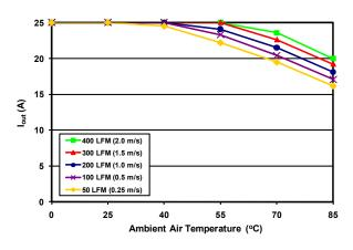
Figure 9: Maximum output power-derating curves vs. ambient air temperature for airflow rates of 50LFM through 400LFM with air flowing from input to output (24V input).
