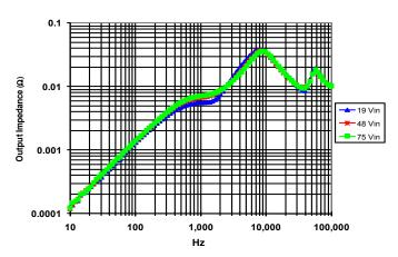
Figure 23: Magnitude of incremental output impedance (Zout = Vout) for minimum, nominal, and maximum input voltage at full rated power.
